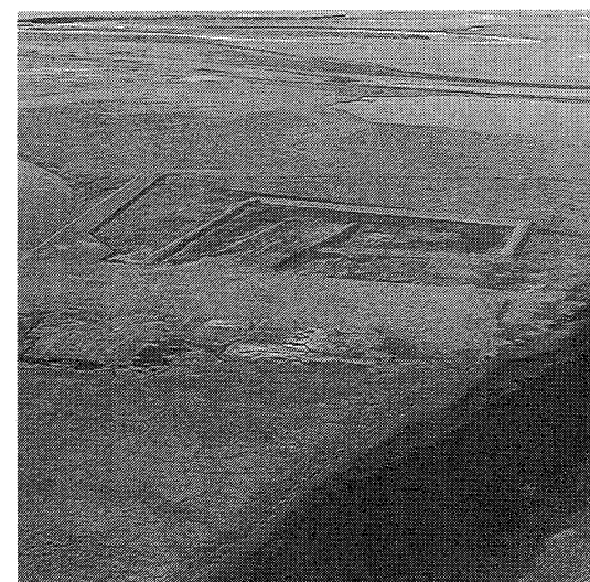
An example of a clean, properly constructed oil drilling pad, located near the mouth of the Iktiklik River. A thick gravel pad and runway complex prevented permafrost degradation during drilling operations.
