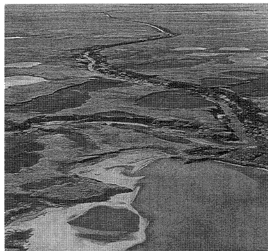
During the late 1940s or early 1950s a trail was bladed east of the Colville delta in winter. Numerous summer thaws since then have slumped and flooded the trail so badly that it has formed a stream, draining several tundra lakes in its path.
